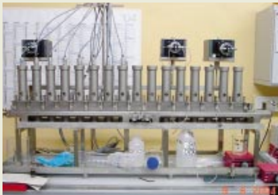
Fig. 1: Set up of the 16 centrifugal extractors installed in the hot cell
