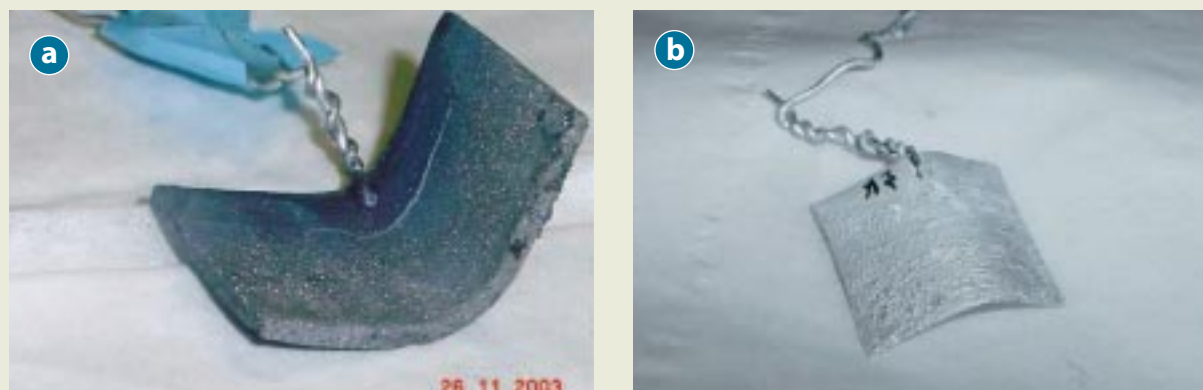
Fig. 2: Al electrode covered with 1.13 g of actinides (a) and the same electrode after treatment in \text{HNO}_3 (b)
